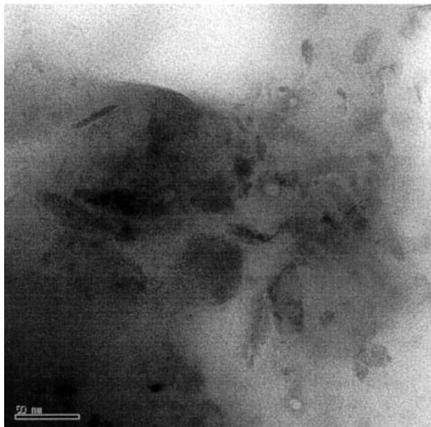
Figure 8 TEM micrographs of nanocomposites (95/5 MAPP/ANMMT).
